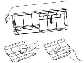
Insert the upper portion of air filter confirming to fit its right and left edges on the indoor unit until it is firmly set.
