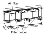
Use a vacuum cleaner to remove the dust from the filters or wash them with water.If you wash the air filters, dry them in the shade.
